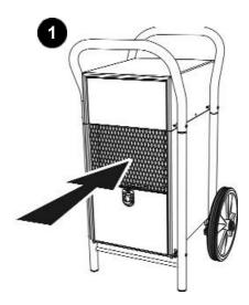
**2. Heavy cleaning:** Open upper door. Remove plastic cleanout by pushing the two locking tabs and lifting. Spray water at coils. Replace the cleanout.
